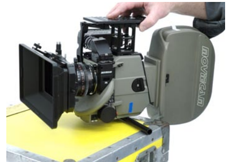
Finding the camera's fore and aft c.g
